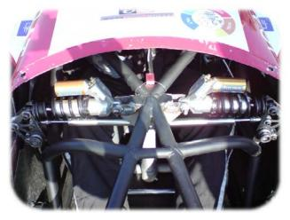
The LVDT displacement sensors will be used as a primary measurement on shock absorber.
